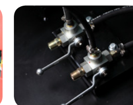
Fuel source switch valve
